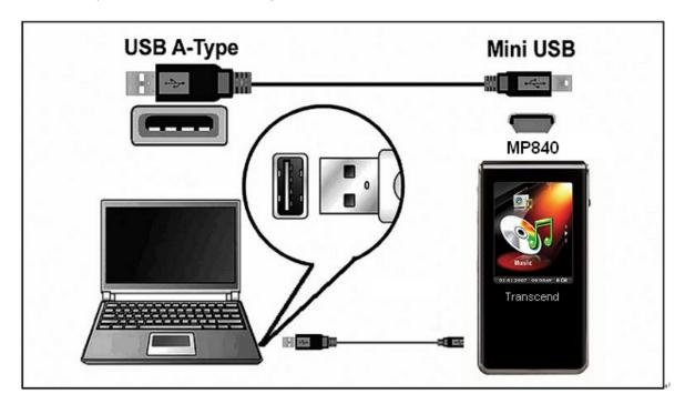
Figure 4. Connecting to a Computer
